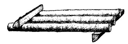
When sawing or drilling wood it is often a problem to hold the piece of wood so that it does not move. This is especially true when a person is working without another person to help. A simple piece of equipment to hold a branch is shown in the diagram above. The following diagram shows this support being used. This is called a bench hook.
