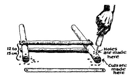
Notches are then made between 3 and 5 cm from the ends of the pieces of wood where the string is to be attached.
