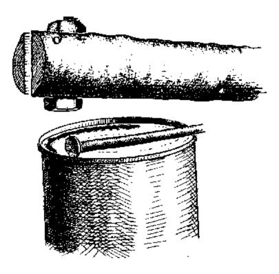
The sharpened edge of the nail is now placed at the edge of the tin, and the other part of the head is hit with a hammer as shown in Diagram D.
