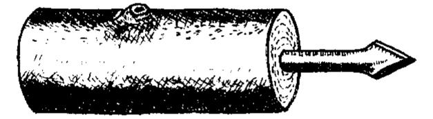
The same procedure can be used to make drills of various sizes, using different sized nails. When using large nails, make sure the wood for the handle is thick enough in diameter so that it will not crack or split when the drill is being used.
