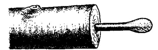
Finally, sharpen the end using a hard stone, or by rubbing it on a hard cement floor until the point looks like this:
