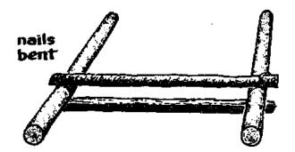
A cut is now made in the ends of the two pieces of wood where the blade is to be attached. The blade should be able to fit into the two cuts without it becoming bent.
