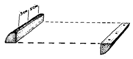
Attach one small piece of wood to the top of one end of the three longer pieces, and the second small piece underneath the other end of the three longer pieces. This can be done by putting a nail into each hole in the short pieces and hammering each nail through and into a long piece. To secure, hammer the points of the nails so they are bent back. The bench hook is then ready for use; it looks like the one shown in the diagram at the beginning of this section.
