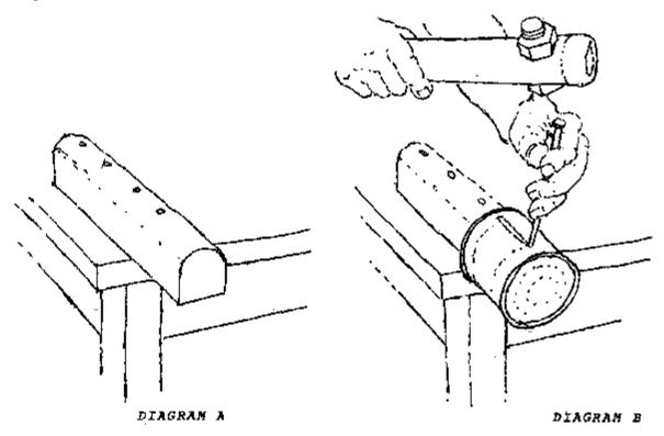
It is also possible to cut a piece of metal from a tin without nailing a pole onto a table. This method, shown below, is much more difficult.
