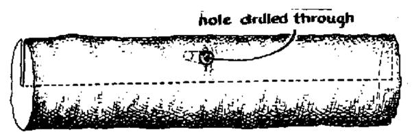
Drill a hole with a small diameter in the middle of the stick as shown. The broken hacksaw blade is inserted into the slot until the hole in the blade is lined up with the hole in the wood. The nail is then inserted. Bend over the nail which sticks out of the other side.
