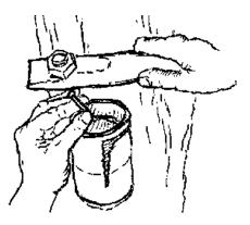
Cutting on a hard surface will damage the point of the chisel. Be sure to place the tin on a wooden surface such as a thick tree branch. When you cut through the tin, the point will go into the wood and the chisel will need to be pulled out before making the next cut.
