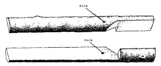
With a drill, make a hole through both pieces. Put a nail through these two holes. Bend the pointed end of the nail. Your tongs are now completed.
