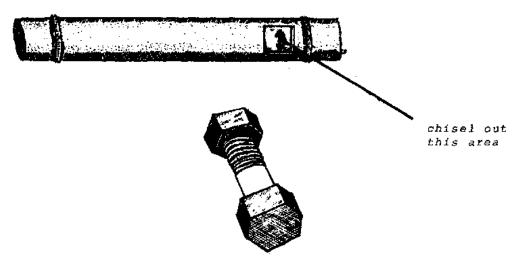
After the bolt has been put through the bamboo handle, and the nut screwed on until the bolt is not loose, the hammer is ready for use.
