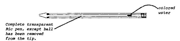
All connections must be sealed, including the small hole on the side of the pen. When the air is warmed and expands, it pushes the colored water. It must not escape elsewhere. The whole device is sensitive to change of temperature. Either the whole thing should be put in the place where temperature is being measured, or the same length must be used for all measurements which are to be compared. It also responds to your warm fingers, and thus must be held some other way.
