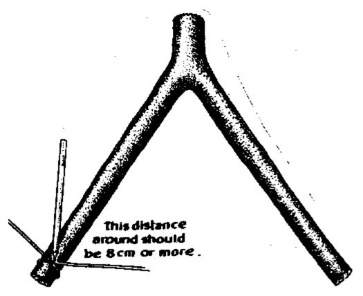
The thinnest part of this piece of wood should be measured to make sure it is thick enough. It should be at least 8 cm around. The wood must be strong enough so that the hacksaw blade remains tight. If the wood is too thin, it will bend when the saw is being used, and the blade will also bend. The blade will last longer the less it bends.
