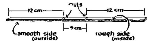
Carefully bend the strip at the two cuts so that the shiny side is inside. With a knife, shave the two ends so that they are thin and come to a point.
