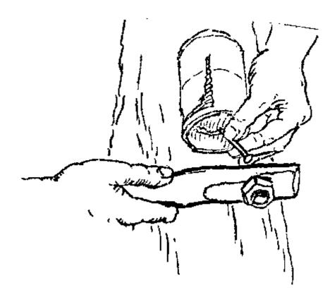
A special tool for cutting the top out of a tin can be made with a 15 cm nail. Rub the head of the nail on a rough stone or rough cement floor until it has the shape shown in Diagram
