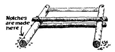
Attach the string by wrapping it around the two pieces of wood at the notches. The string should be wrapped 2 or 3 times and then tied together. Put the last piece of wood through the string and turn until the string twists enough to tighten the blade.
