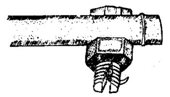
In cutting the bolt with the hacksaw, first make a vertical cut about 1 cm deep. Then cut between 2 and 3 mm away from the first cut. (mm - millimeter; a millimeter is one tenth of a centimeter.) This second cut should be a diagonal one. It is important that the cut be made no larger than 3 mm. If the cut is wider, it will be diffecult to remove any nails.
