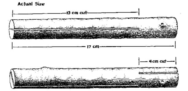
Use your chisel and hammer to chip away at point "A" as shown in the diagram. Chisel a little away at a time. Do this until the cuts are connected. Turn the branch over and do the same thing to connect the two cuts on the other side.
