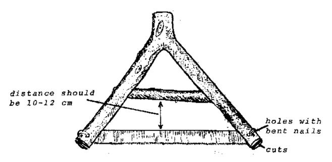
Next, hammer a 4 cm nail through one side of the piece of wood and into the end of the straight piece of wood as shown in the diagram at A. Pull the short piece of wood upwards to tighten the blade and hammer the smaller nail (2 or 3 cm) Just below the end of the short piece as shown in the diagram at B.
