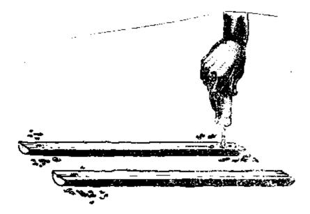
The drill also can be used to prepare a piece of wood for a nail. If a hole is made in a piece of wood before a nail is pounded into it, the wood will be less likely to split. Choose a drill which will make a hole that is slightly smaller in diameter than the nail that you want to use. Drill the hole not quite through the other end. When joining two pieces of wood, do this for both pieces. Then bang the nail through the holes in the two pieces.
