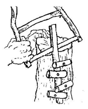
Now remove the branch from the wood holders. Cut off the extra wood at the other end, so your piece is 17 cm long. Again, hold the branch with wood holders this time with the end with the 13 cm cut down. The end that is up should now be cut to a depth of 4 cm at right angles to the 13 cm cut. The diagrams illustrate these cuts.
