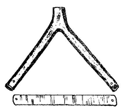
The hacksaw blade is used to make a cut in each end of the piece of wood. These cuts should be aligned with each other so that the blade can be placed into the cuts without becoming bent. The cuts should be about as deep as the width of the blade.
