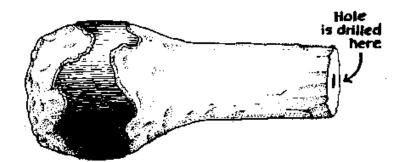
Use a drill that will make a hole a little smaller than the nail. Make a hole in the end of the handle as deep as it is possible to make with the drill. Use the saw to cut the nail near the head of the nail, as shown in the diagram.
