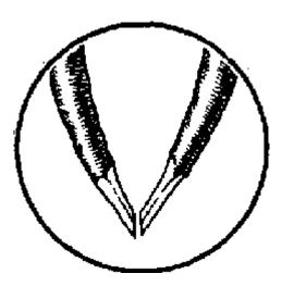
With a sharp knife, cut the ends so that they are thin and tapered. Any small object, such as a nail or pin, can be picked up.
